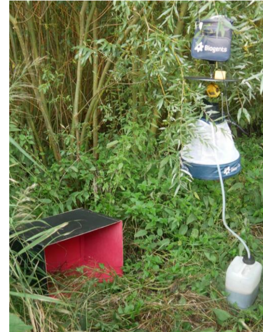
Mosquito trapping on bird ringing sites - molasses fermentation-baited BG-pro traps
